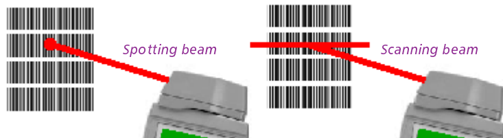
Figure 2-9: Long-Range Laser Operation in the Falcon 310 , 315 , 320 , and 325
